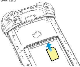
Insert a memory card with the gold-coloured contacts facing downwards. Push the memory card into the slot until it locks in place.
