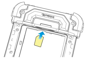
Insert a memory card with the gold-coloured contacts facing downwards. Push the memory card into the slot until it locks in place.
