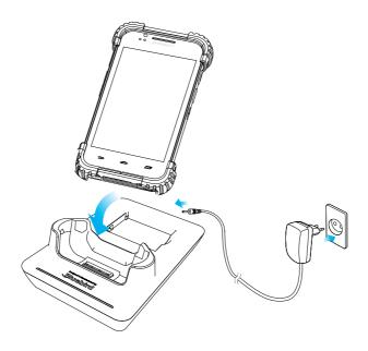
As you see in the picture, connect the adapter with the power cable to charge the device.
