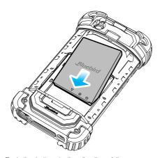
Push the battery to the direction of the arrow.
