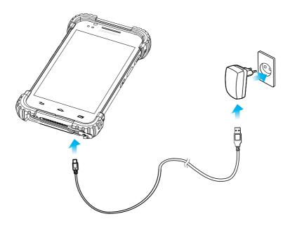
Plug the small end of the cable into the micro USB port on the device and plug the normal USB connector of cable into an charger.
